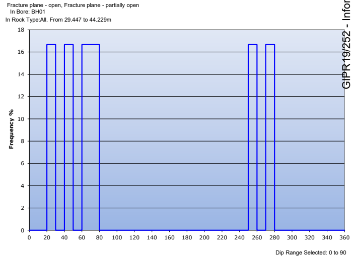
Figure 9 BH01 TOP fractures dip directions histogram
