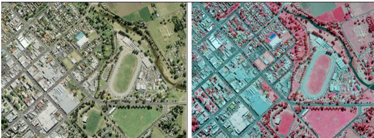
Images depict samples of airborne imagery over Bathurst, NSW (left) at 10cm in RGB and CIR (Left) © Spatial Services 2018
