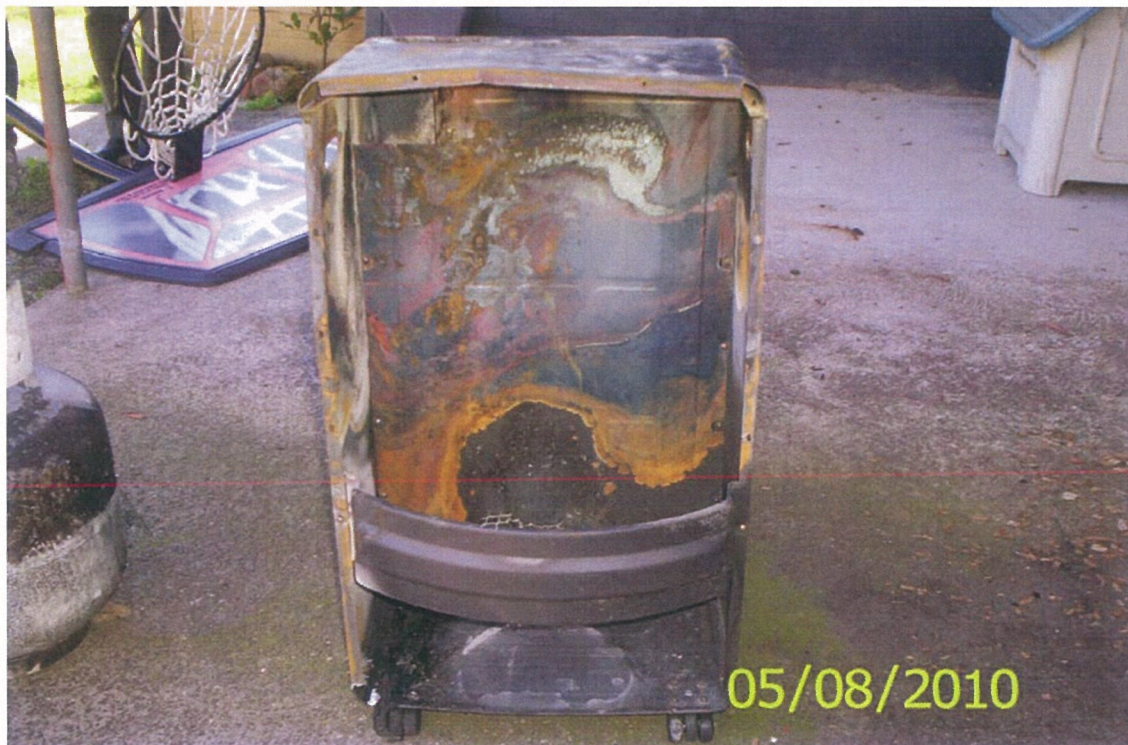
Fire damage to LPG Cabinet Heater (rear view)
