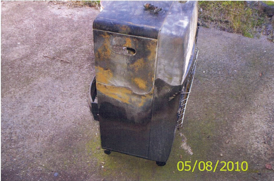
Fire damage to LPG Cabinet Heater (side view)
