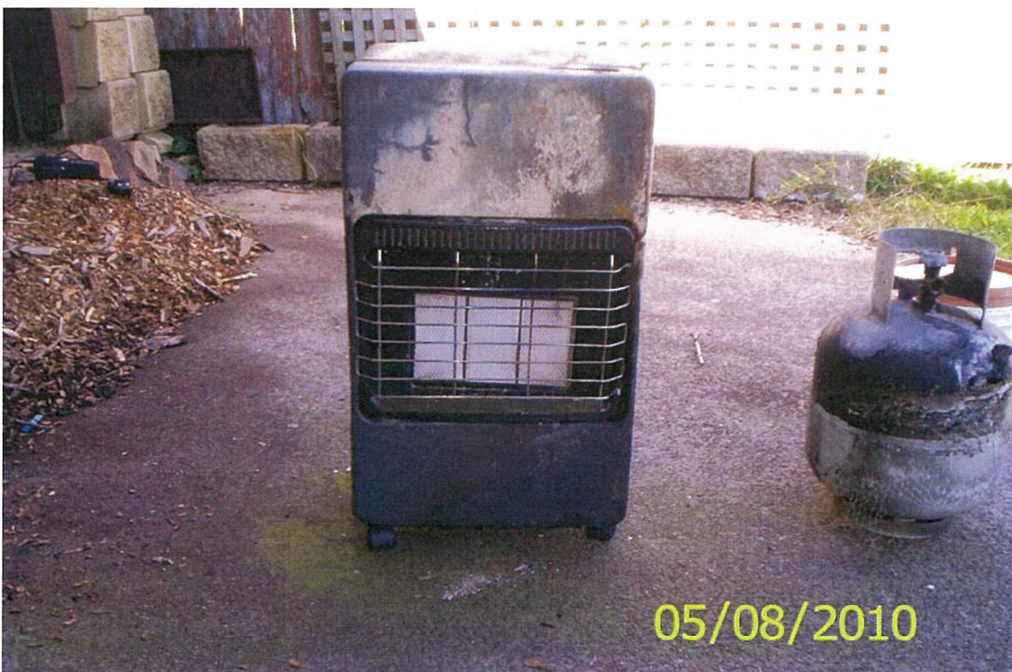
Fire damage to LPG Cabinet Heater (front view) and LPG cylinder
