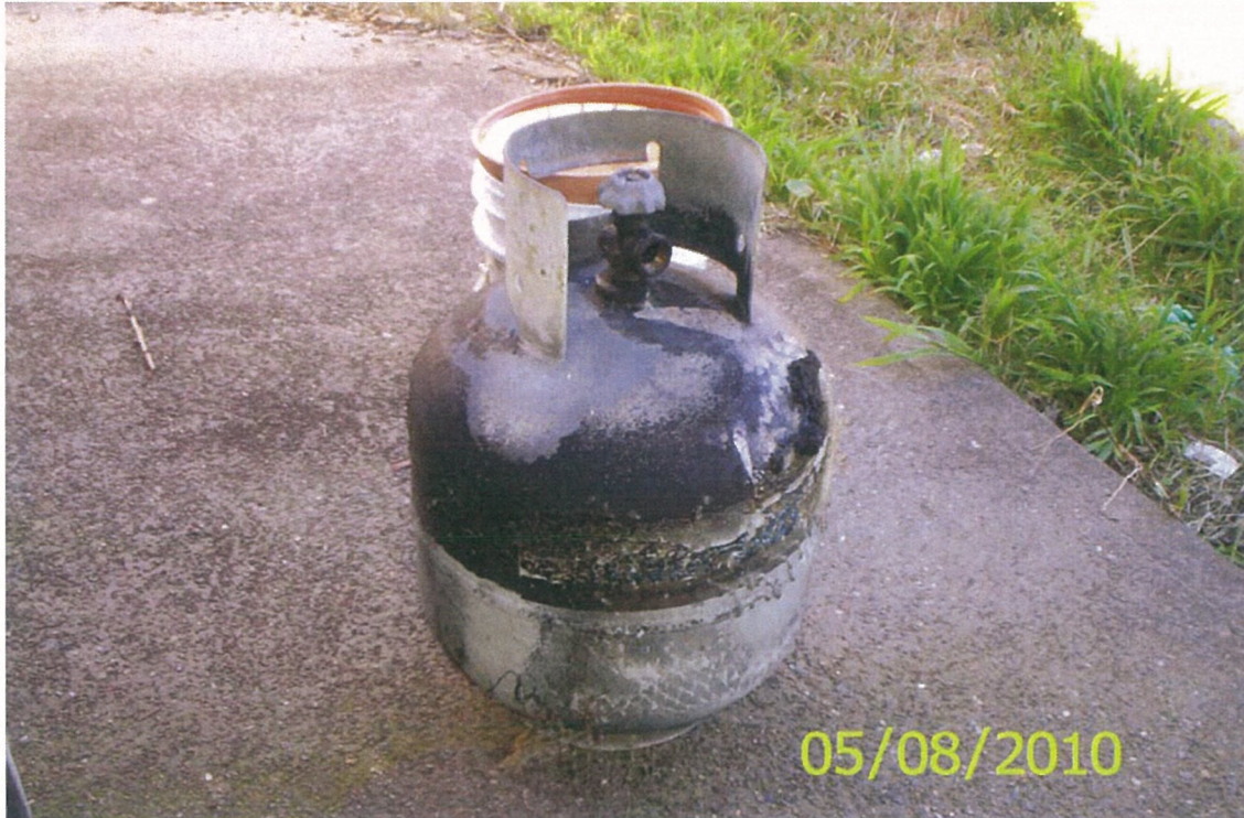
Fire damage to LPG cylinder (normally attached to Cabinet Heater)
