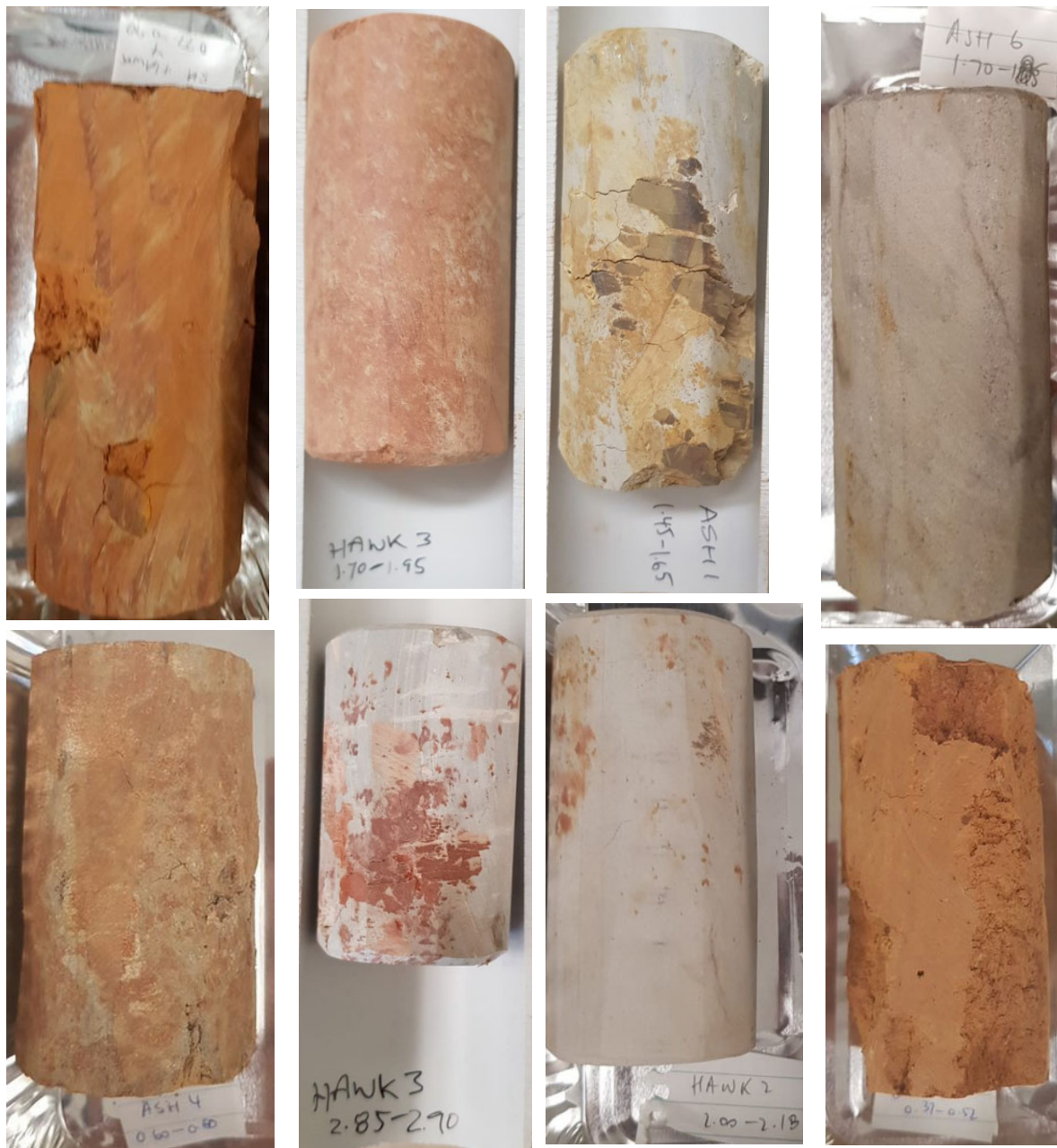
Figure 8: Typical shrinkage cores after cutting and shaping with a diamond saw
