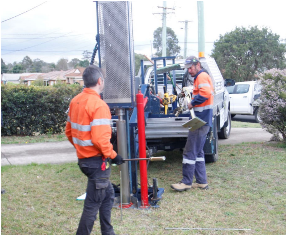
Figure 3: Sampling operation using the Grace Coring rig.
